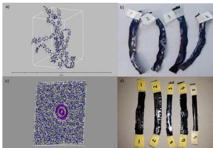
Figure 1: a) simulated ABPBI cell, b) ABPBI sample, c) ABPBI carbon nanotube composite simulated cell, d) ABPBI carbon nanotube composite sample
